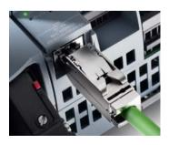
The integrated PROFINET interface is used for programming, as well as for HMI and PLC-to-PLC communication. Additionally, it supports communication with third-party devices using open Ethernet protocols. This interface features an RJ45 connector with auto-cross-over functionality and provides for data transmis-sion rates at 10/100 Mbit/s. It supports up to 16 Ethernet connections and the following protocols: TCP/IP native, ISO on TCP, and S7 communication.
