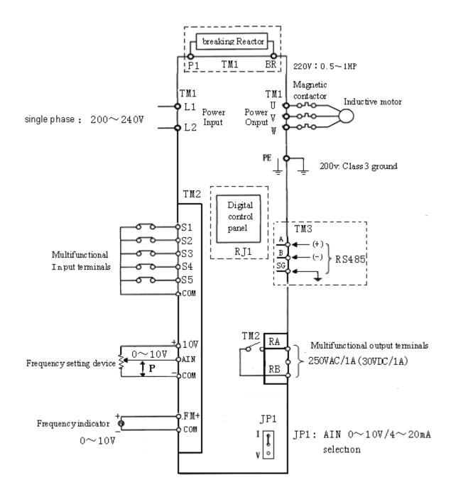
Figure 3-7 Wiring Diagram
